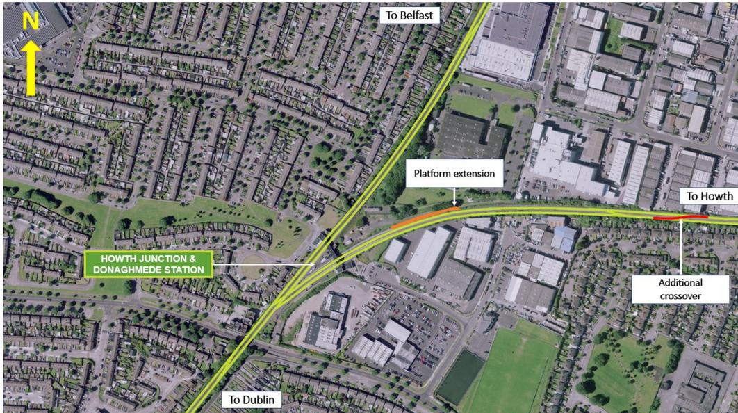
**Figure 5-9: Aerial view of Option 5 (green indicates existing track and red indicates new track)**
