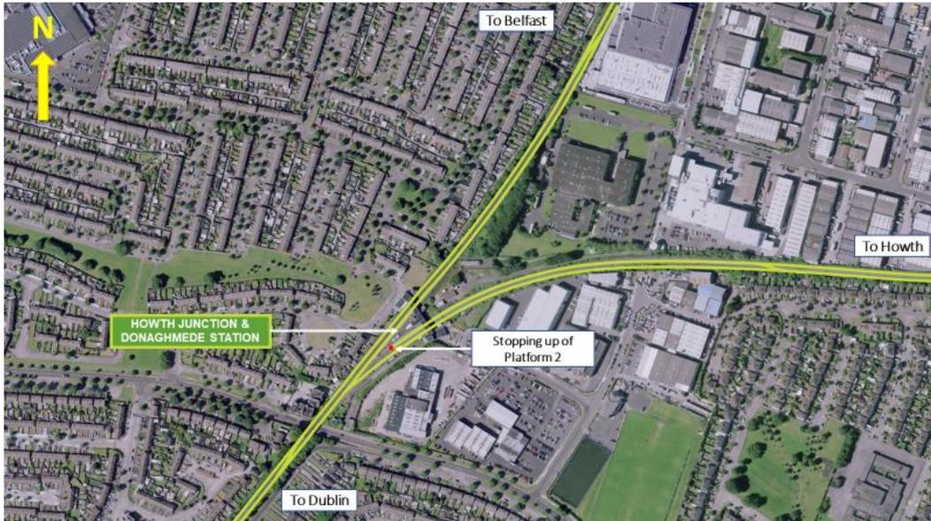
Figure 5-7: Aerial view of Option 4 (green indicates existing track and red indicates new track)
