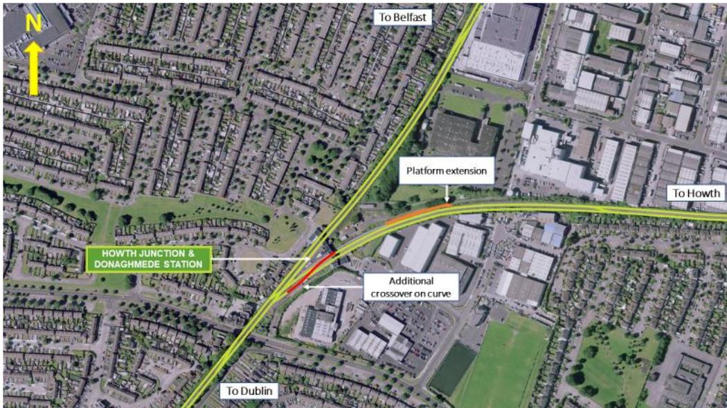
Figure 5-5: Aerial view of Option 3 (green indicates existing track and red indicates new track)
