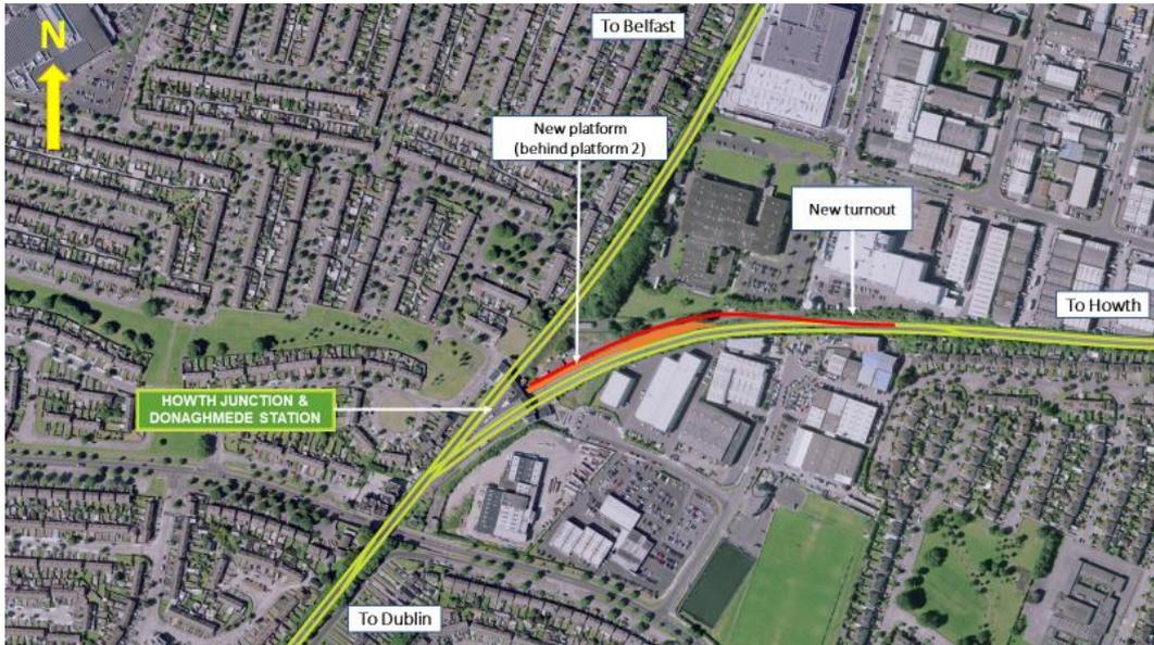
Figure 5-15: Aerial view of Option 7a (blue indicates existing track and red indicates new track)
