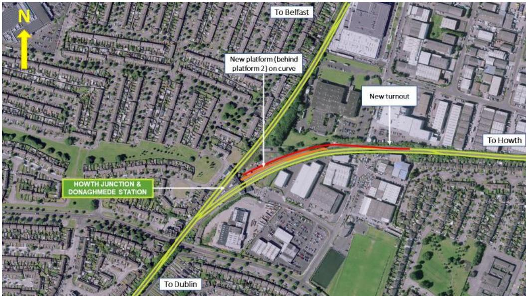
Figure 5-11: Aerial view of Option 6 (green indicates existing track and red indicates new track)
