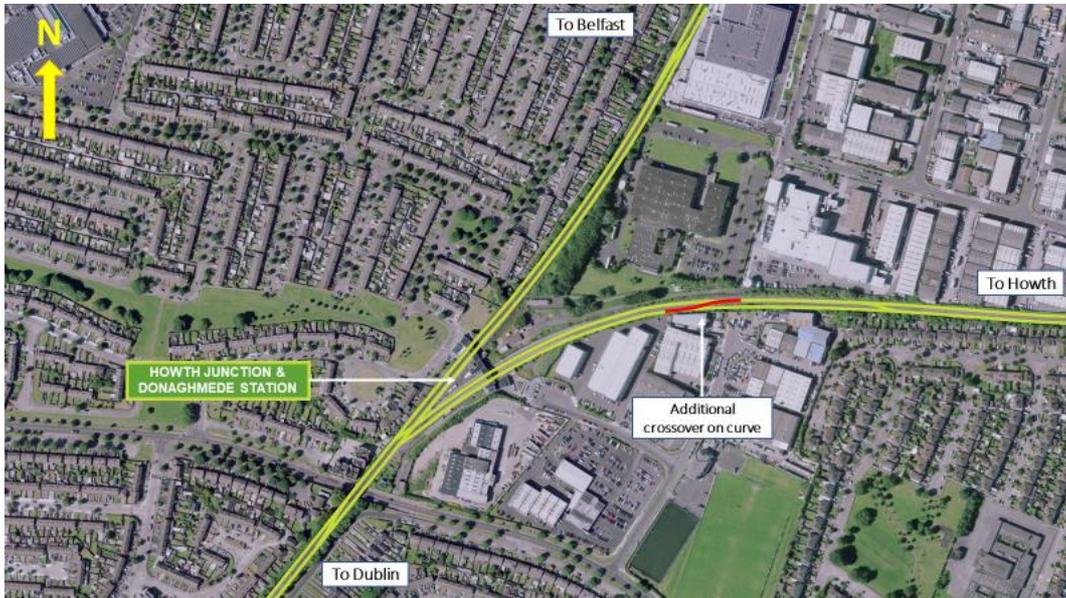
Figure 5-3: Aerial view of Option 2 (green indicates existing track and red indicates new track)
